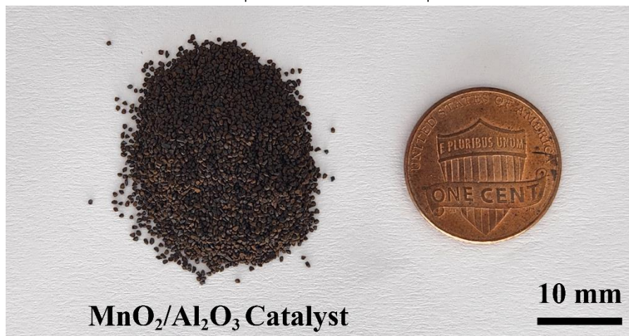
Fig. 2. Fabricated \text{MnO}_2/\text{Al}_2\text{O}_3 catalyst with a support mesh size of 35–40, 425\text{--}500 \mu\text{m}
