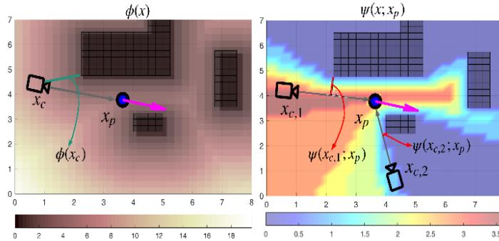
**Fig. 3 Score for safety (left) and visibility of  $x_p$  (right) fields with colorbars.**
