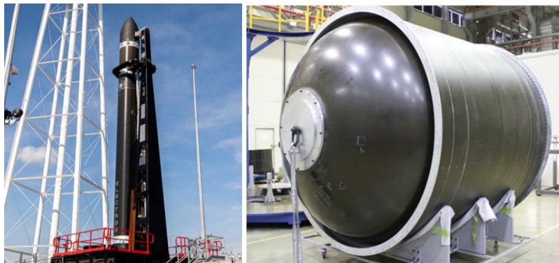
Fig. 2 Rocket Lab's Electron (left) and ANH Structure's composite propellant tank (right)
