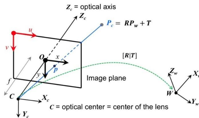
Fig. 7. A 3-D point and the camera, from the world coordinate system.
