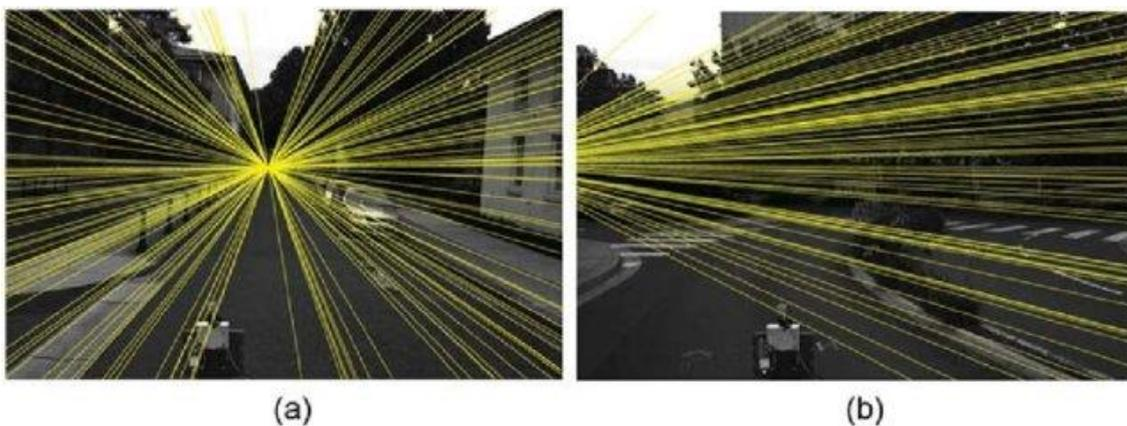
Fig. 12. Epilines for video frames taken while camera translation(left) and rotation(right) (32).
