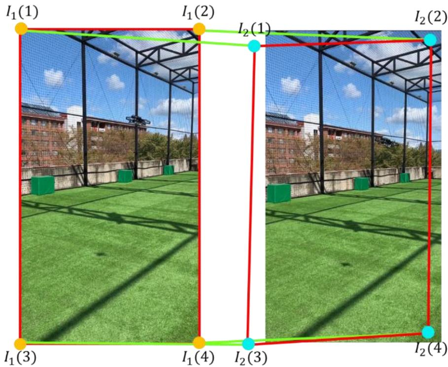
$$[I_1(1) \ I_1(2) \ I_1(3) \ I_1(4)] = \begin{bmatrix} h_{11} & h_{12} & h_{13} \\ h_{21} & h_{22} & h_{23} \\ h_{31} & h_{32} & h_{33} \end{bmatrix} \cdot [I_2(1) \ I_2(2) \ I_2(3) \ I_2(4)]$$
