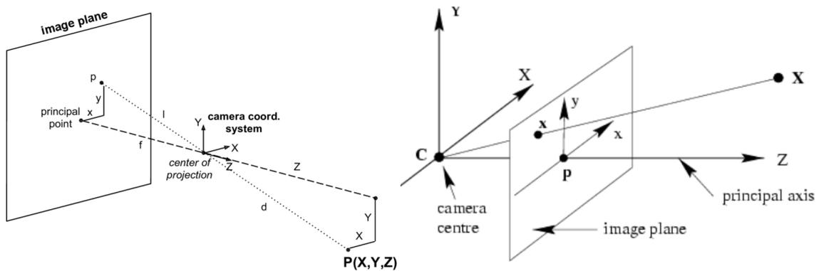
Fig. 5. The standard pinhole camera model(left), and the pinhole camera model with the image plane in front of the center of projection(right)
