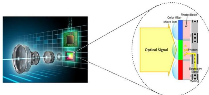
Fig. 4. Image formation of a digital camera
