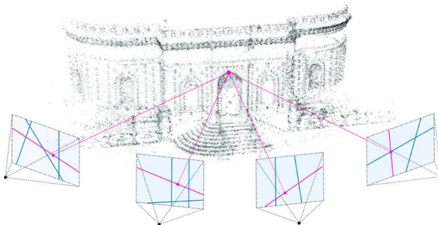
Fig. 9. Structure from Motion(SfM)
