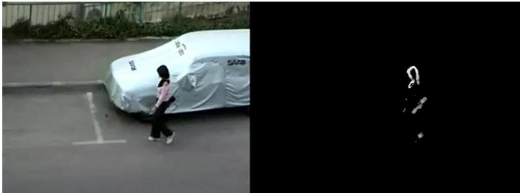
Fig. 22. Original video frame(left) and background subtracted result(right)
