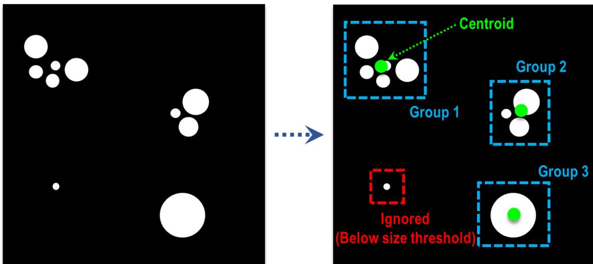
Fig. 27. Clustering procedure of the modified DBSCAN algorithm
