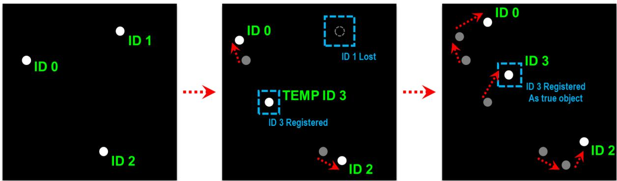
Fig. 28. Tracking procedure of the distance–based tracking algorithm
