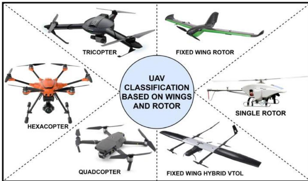
Fig. 1. Various body types of UAVs <sup>(5)</sup>
