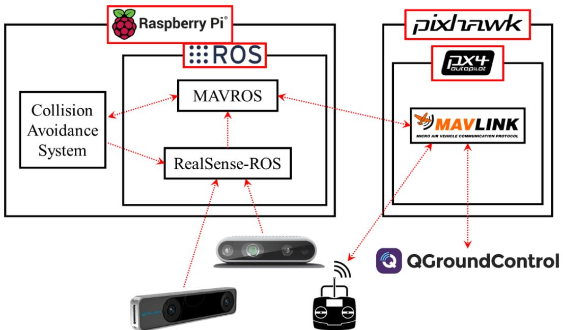
Fig. 34. A schematic diagram of the system.
