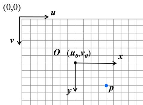
Fig. 6. The 2-D image plane coordinates(x, y)and pixel coordinates(u, v).
