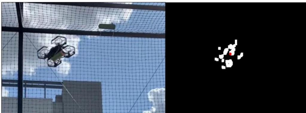
Fig. 25. A single moving object shows up as “blobs” after these operations.
