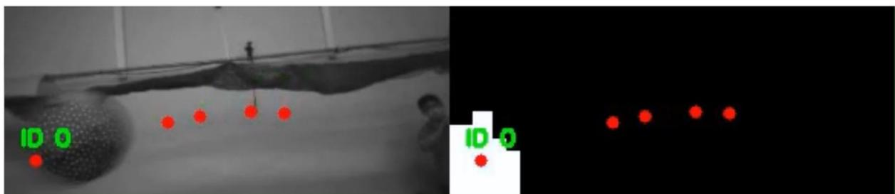
Fig. 37. Detection and tracking a flying ball
