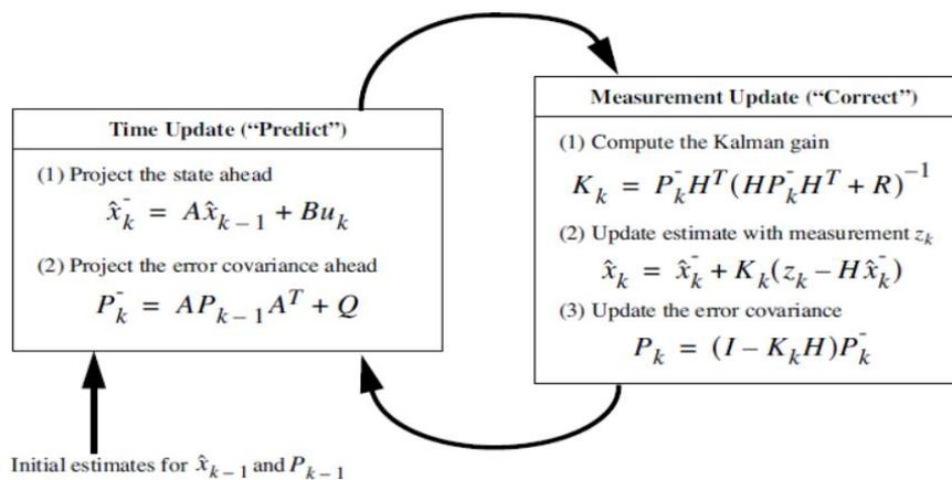
Fig. 30. The recursive operation of the Kalman filter
