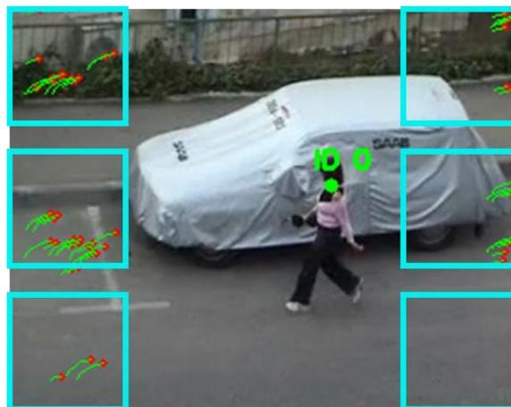
Fig. 20. Six boundary regions where optical flow is calculated
