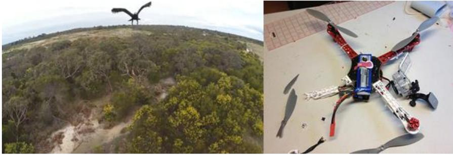
Fig. 3. A crashed multi-rotor UAV after a mid-air collision with an eagle.
