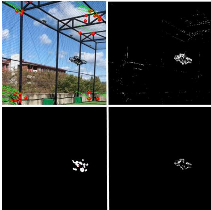
Fig. 24. (From upper left, clockwise) The original frame / background subtracted frame / median filtered frame / dilation filtered and binarized frame
