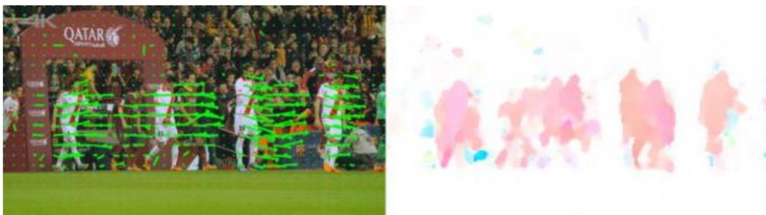
Fig. 14. Lucas-Kanade(left) and Horn-Schunck(right) algorithms in operation
