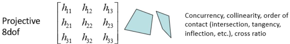
Fig. 12. The projective transformation maps an arbitrary quadrangle into another quadrangle.
