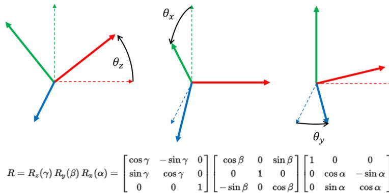
Fig. 8. Compositions of a standard rotation matrix
