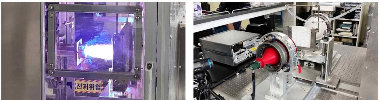
Fig 15 High temperature free space measurement plasma equipment
