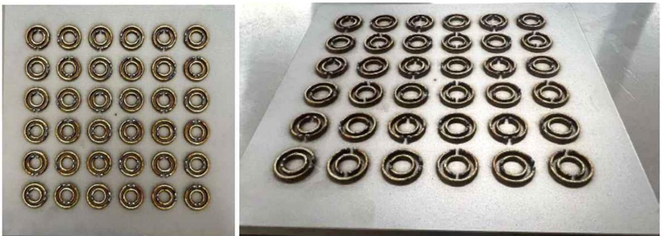
Fig 10 3D printed specimen after fabrication
