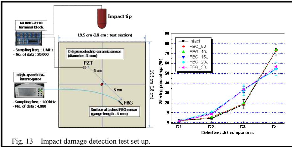
Fig. 13 Impact damage detection test set up.
